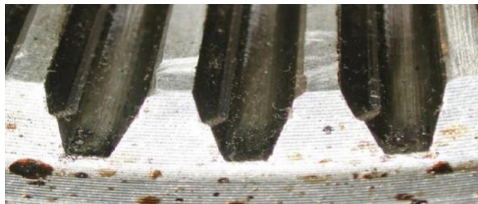
Figure I-11 : Usure abrasive "Engrenages". [15]
