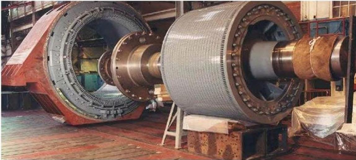
**Figure I.7 :** Machine asynchrone de 4.7MW, 45tr/min.
