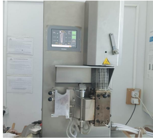
Figure IV. 7. L'extrudeuse bis-vis de type 15cc Twin Screw Compounder
