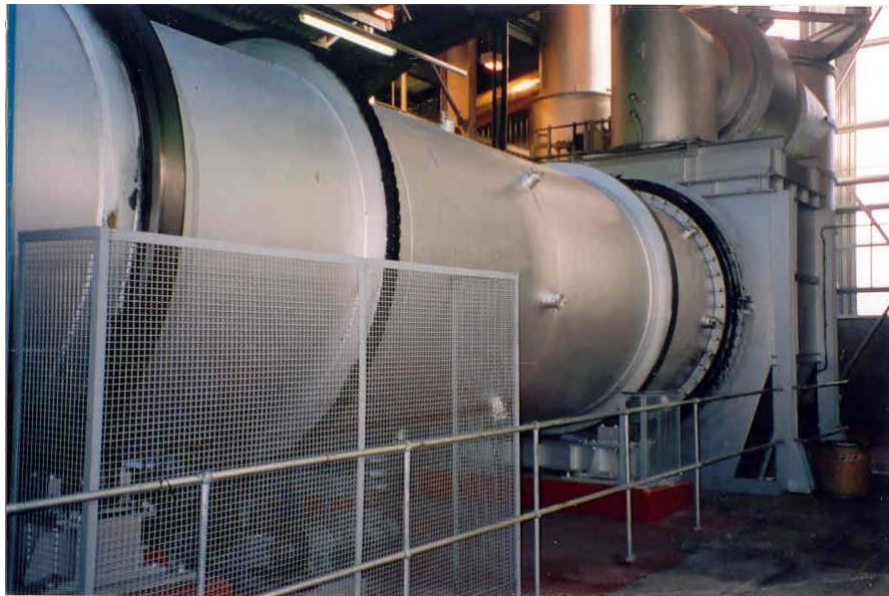
Figure 1.6: Incinérateur four rotatif FRCD 450 (Walter,2010).
