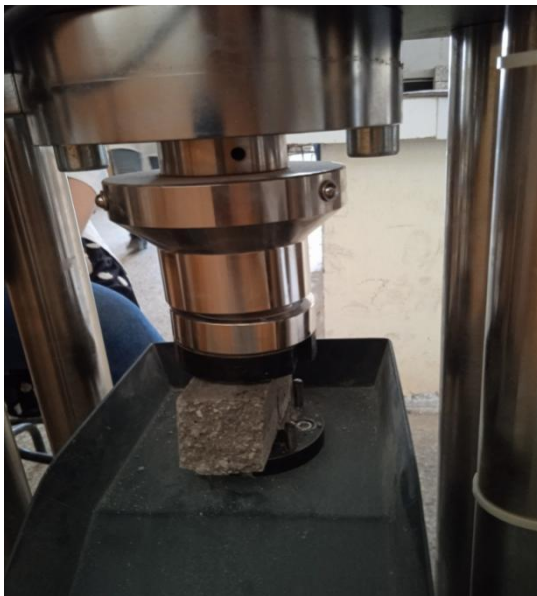
Figure III.27: Essai de compression
