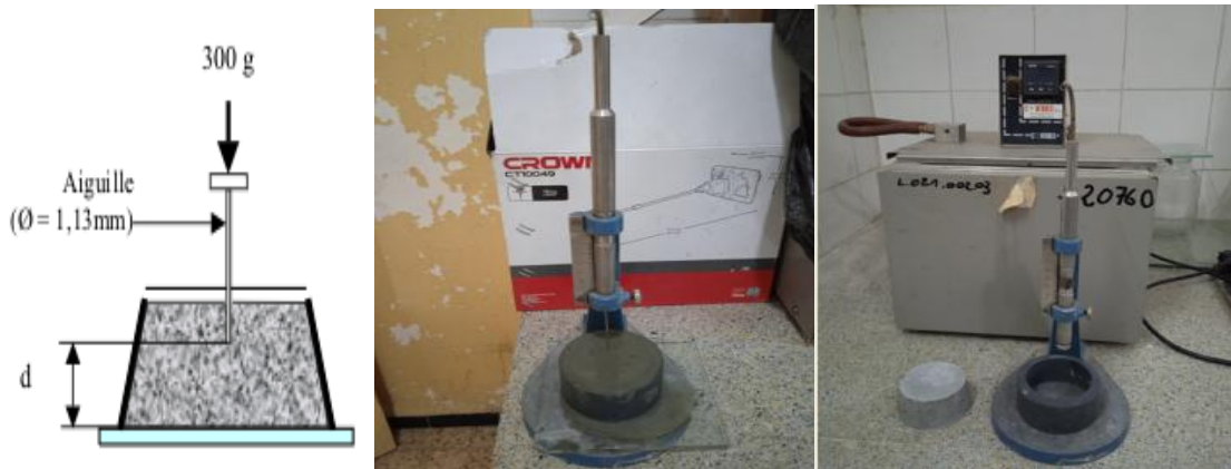
Figure II.13 : Essai de prise
