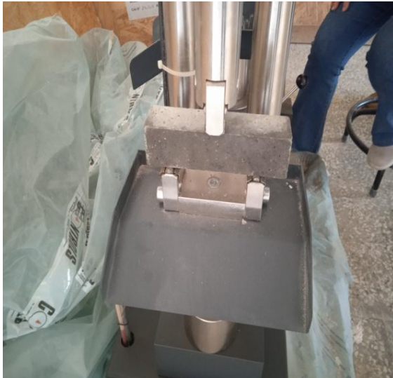
Figure III.23: Essai à la flexion
