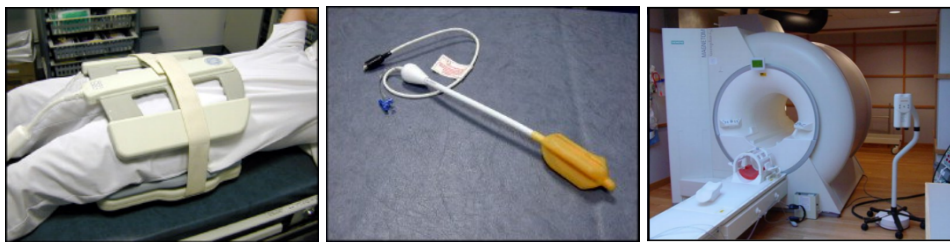
(A) Pelvic coil (B) Endorectal coil (C) Siemens 1.5T MRI FIGURE 1.7 – Used for some of the MRI-MP acquisitions. Adapted from Niaf [1].
