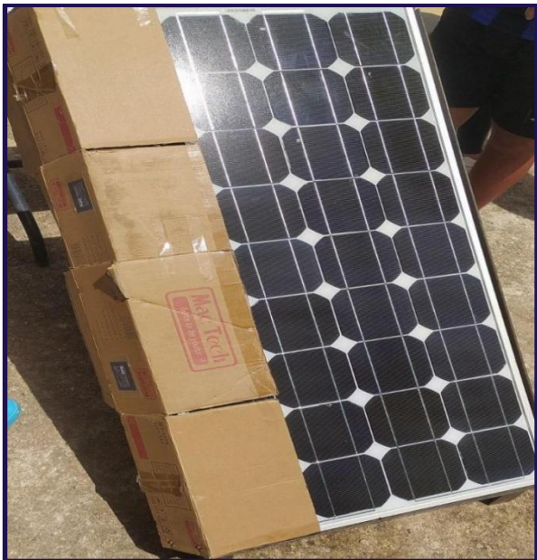
Figure 32: Clean panel, shading 25%
