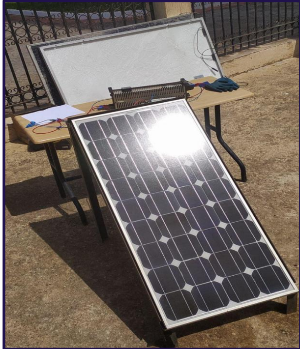
Figure 31: Clean panel, shading 0%
