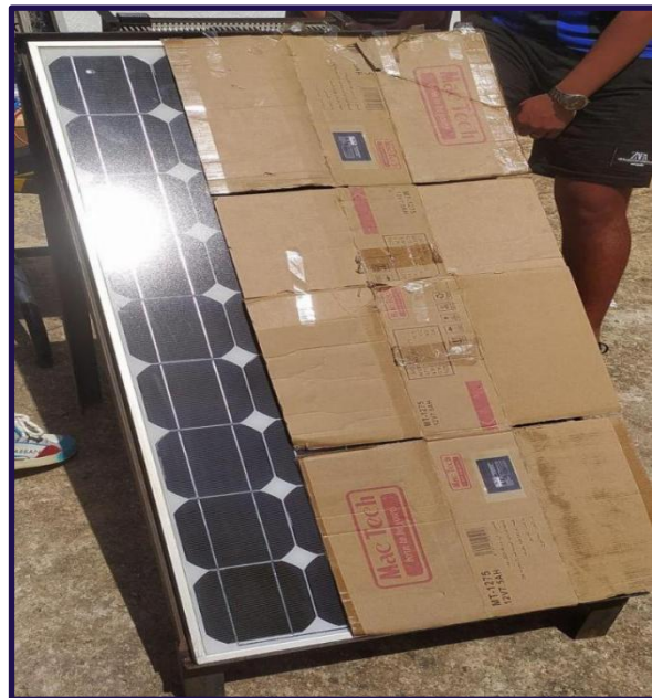
Figure 33: Clean panel, shading 68%
