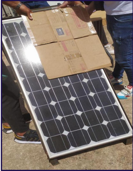
Figure 30: Clean panel, shading 34%
