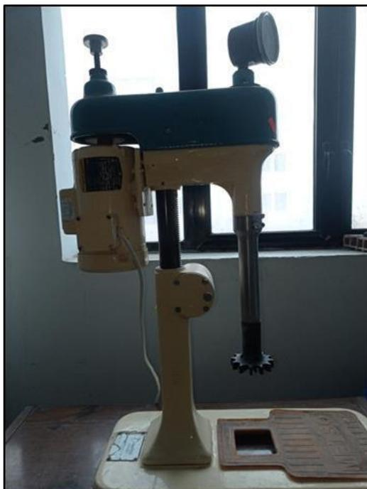
**Figure IV.2:** Cellule de flottation LTM GP.
