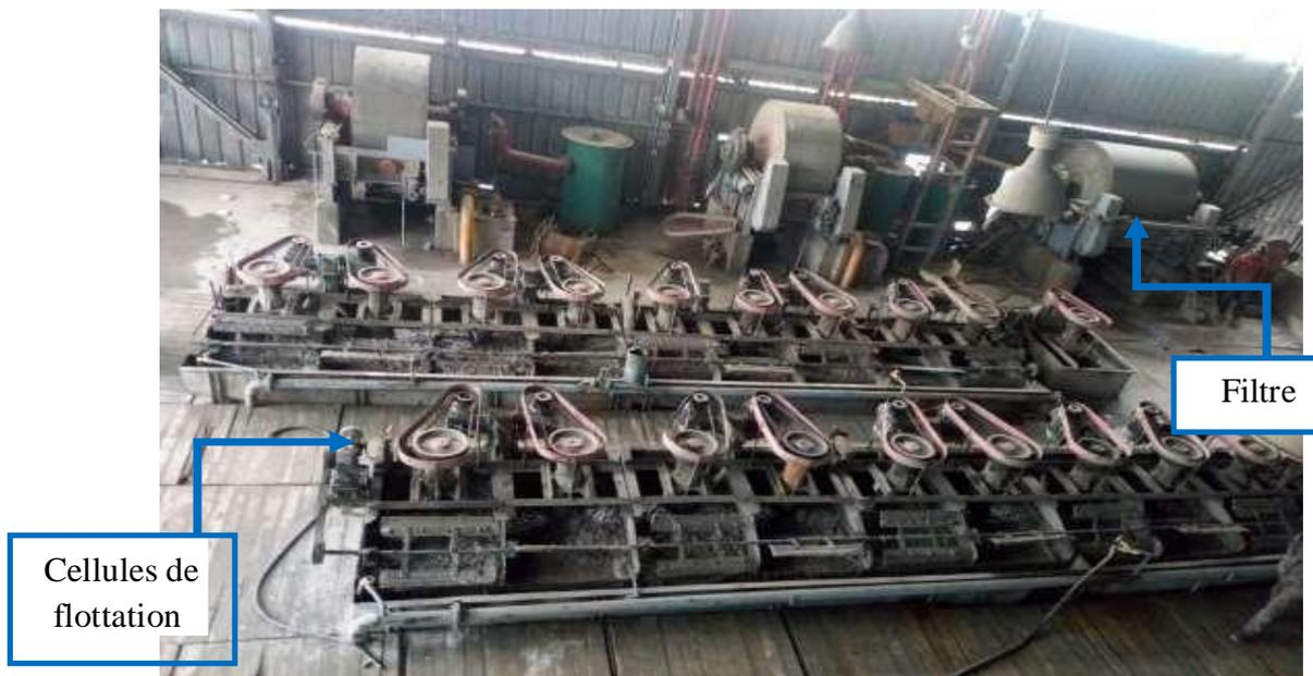
Figure II .9: Section flottation - filtration.
