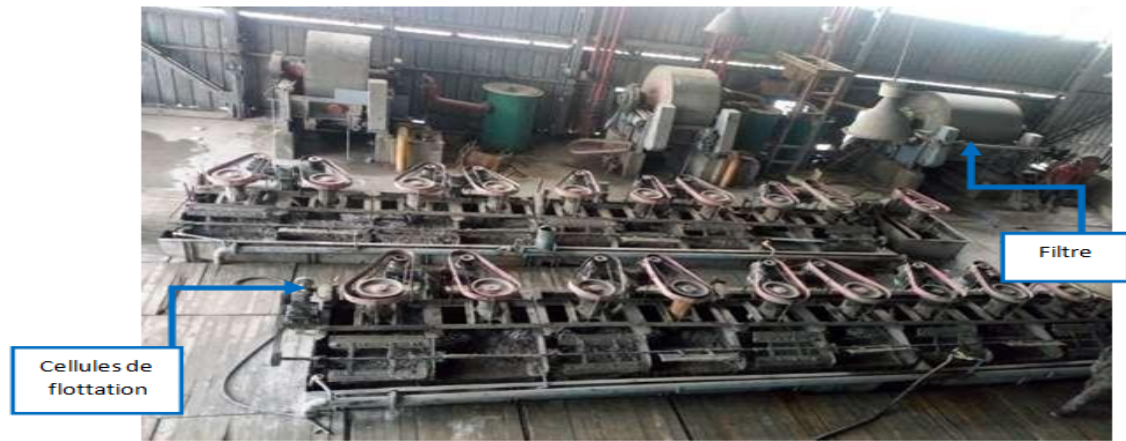
FIGURE 1.11 – Section flottation – filtration
