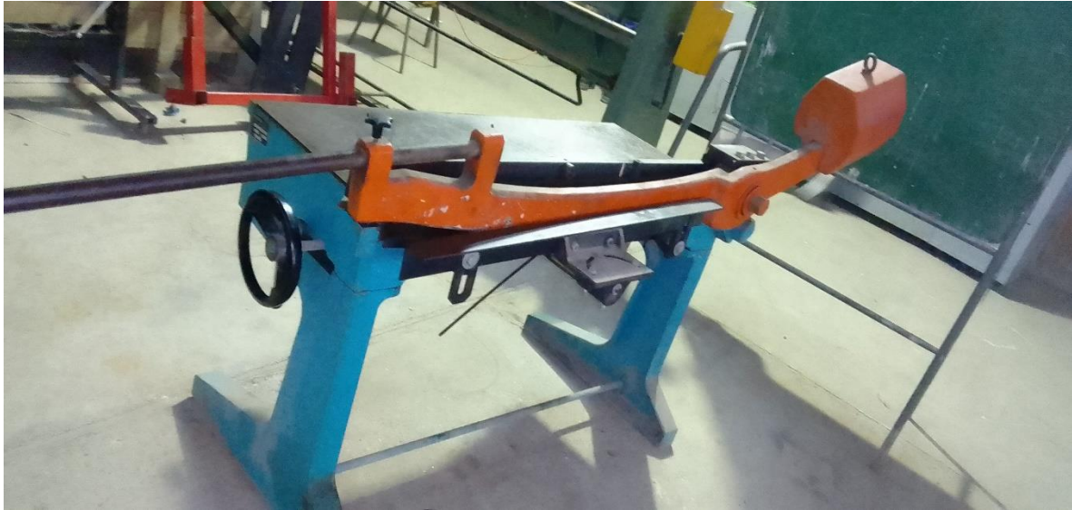
Figure II.2 : Cisaille guillotine manuelle KHS e 1000.
