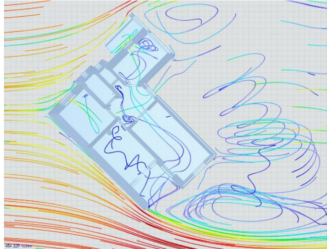
Figure 3.60 : Effect of prevailing winds on the Sidi Ali Lehber house (Source: RWIND, 2023)
