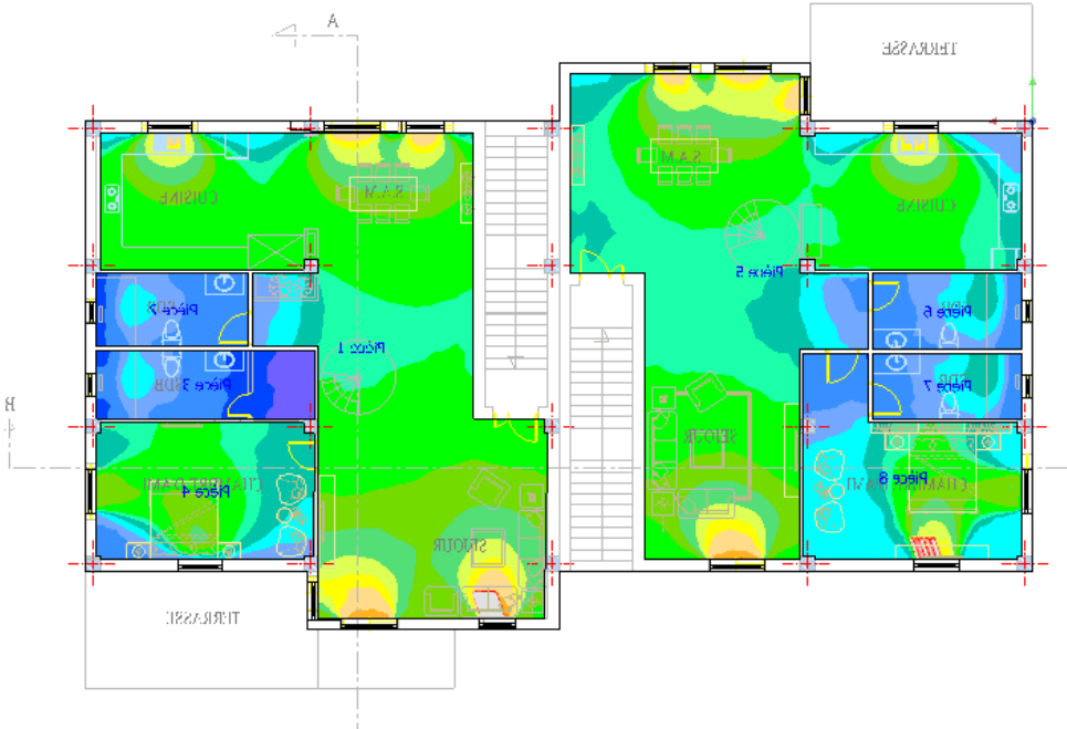
Figure 4.68 : Simulation verification of the semi-collective house in mid-season at noon (Source: DialuxEvo, 2024)
