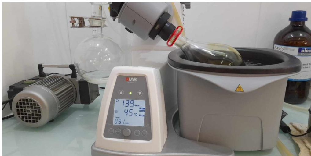
Figure 7 : Evaporating the ethanol from the extract using the rotary vacuum evaporator
