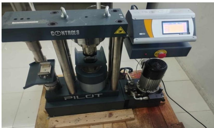
Figure III.5 : Presse hydraulique type CONTROLS PILOT PRO.
