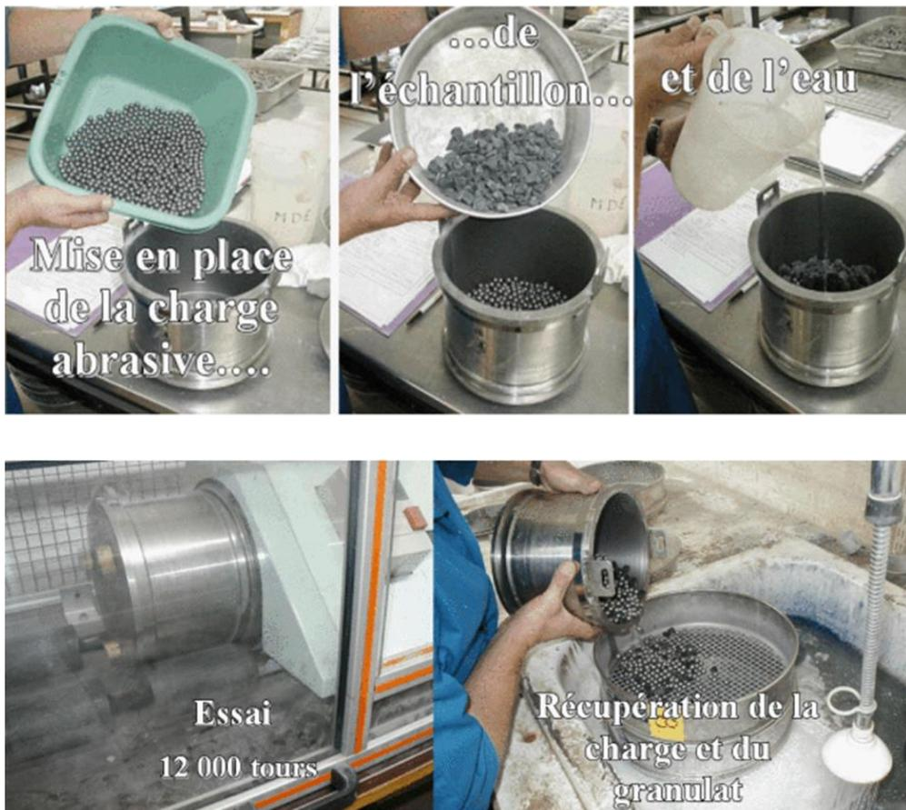
Figure II.6: L'essai Micro-Deval
