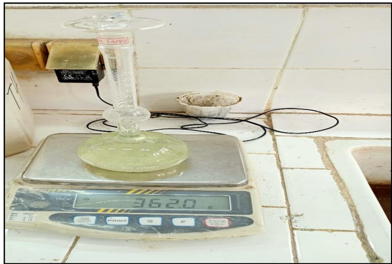
Figure II.15 Chatelier masse M1.
