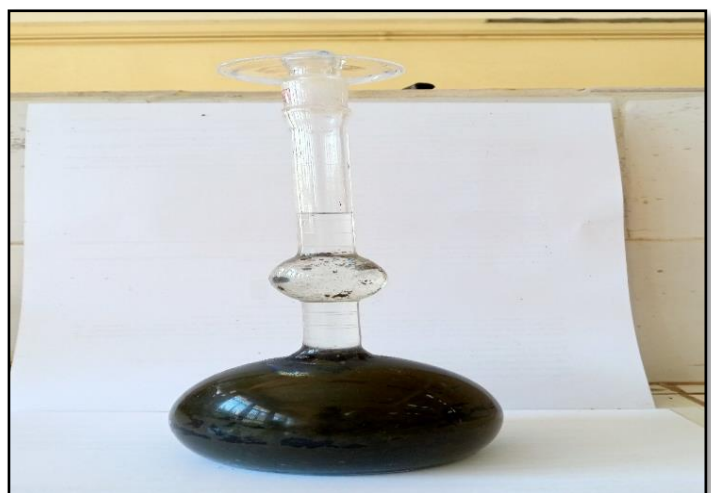
Figure II.16 Chatelier masse M2.
