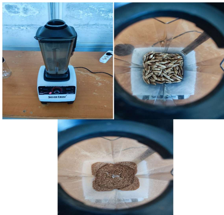
Figure 3 : Photography showing the different blending steps using a 3000 Watts rotator blender
