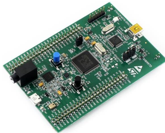
Figure 2-26 STM32F407 DISCOVERY board.
