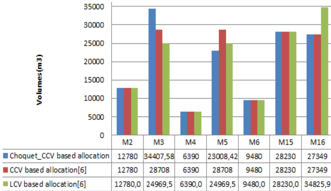
Figure 4.11 – Volumes allocated to mills processing SPF species obtained based on the Choquet-CCV method, the CCV and the LCV
