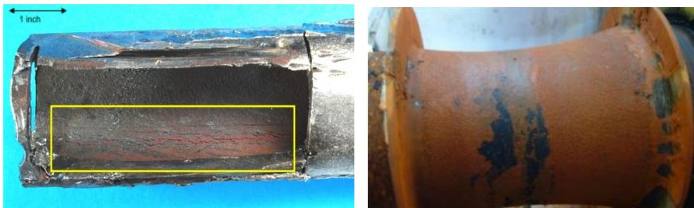
**Figure I.17 :** Corrosion fatigue
