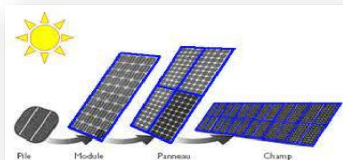
Figure I.14: Cellule, module, panneau, champ photovoltaïque
