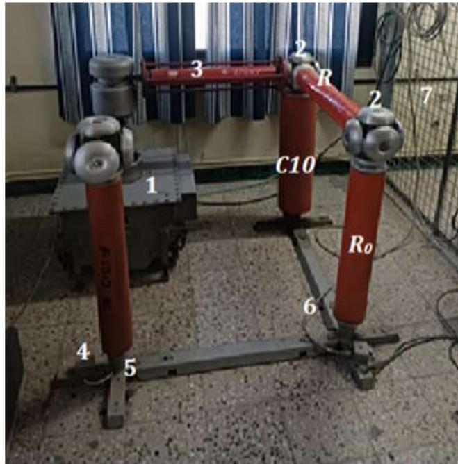
Figure II 2: Photo de la source haute tension continue
