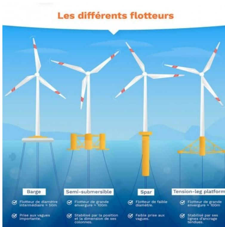
Figure I. 9: Eolienne flottante [12].
