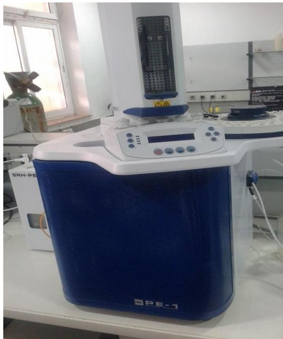
**Figure 40:** NIC Mercury Analyzer (P E - 1)
