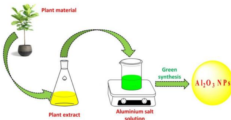
Figure 5. Schematic representation of green synthesis of \text{Al}_2\text{O}_3 NPs
