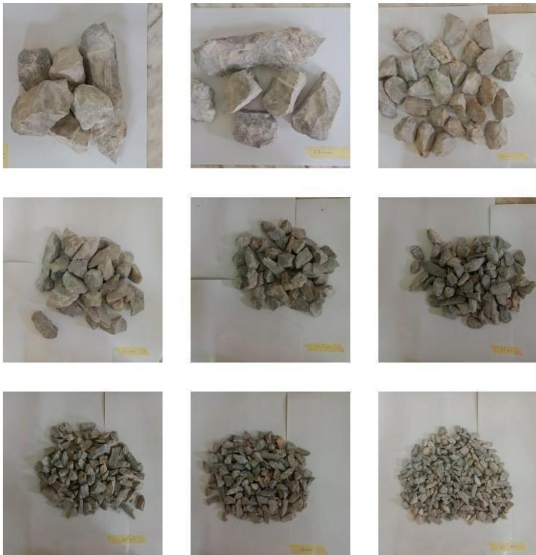
**Figure III.8:** Classification obtenu (80 mm - 12.5mm).
