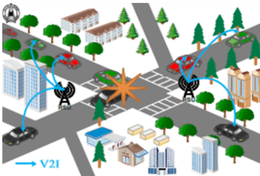
FIGURE 1.4 – Exemple de communication V2I[10]
