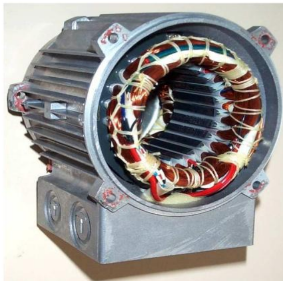
Figure I.2: Stator d'une machine asynchrone [19].
