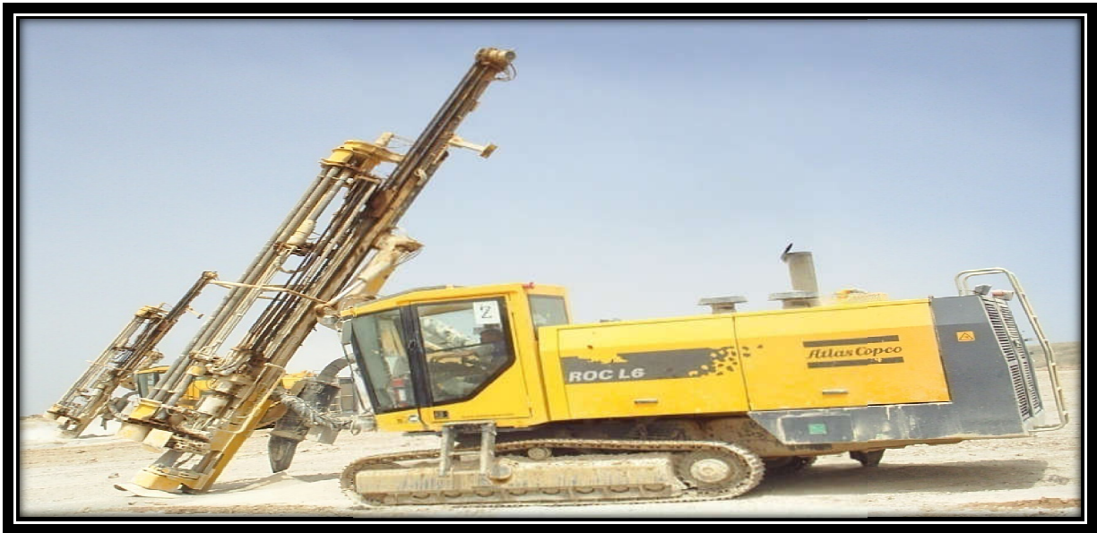
Figure III.1 : Sondeuse ATLAS COPCO ROC L6.
