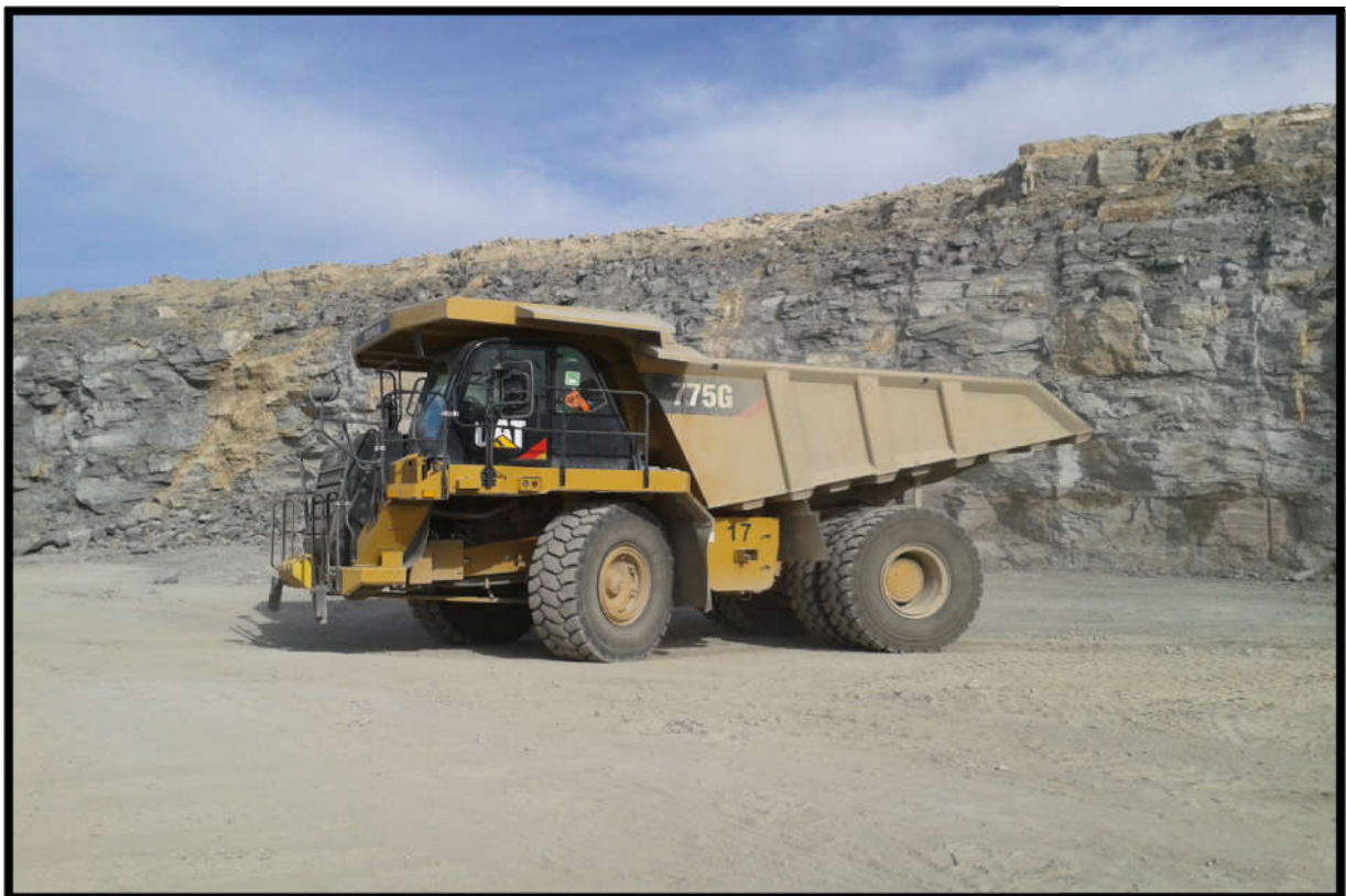
Figure IV.3: Dumper CAT 775. (prise le 14/03/2017)
