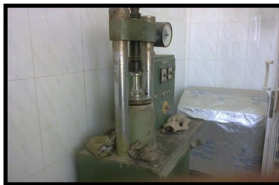
Figure III.5 : Appareil à compression.
