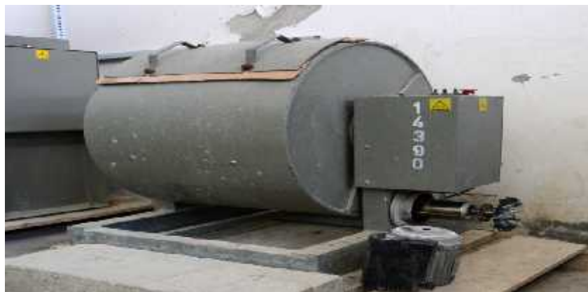
Figure II.11 : Machine Los Angeles [65].
