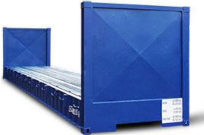
Figure n°04 : le conteneur flat rack
