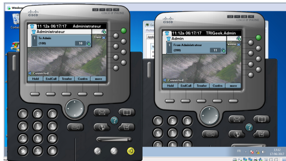
FIGURE 4.2 – Appel entre deux softphone Cisco IP Communicator.
