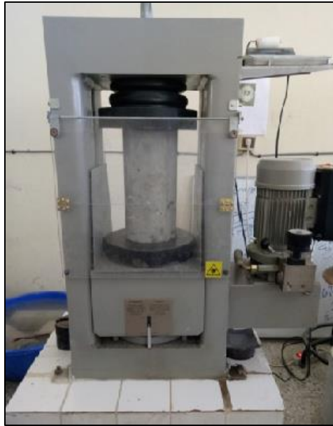
Figure II.26 : Essai de compression.
