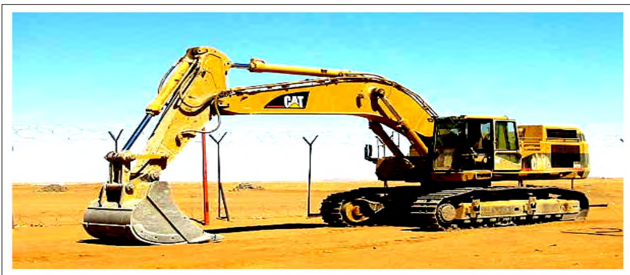
Figure II.9 : Pelle hydraulique-CATERPILLAR 365BL
