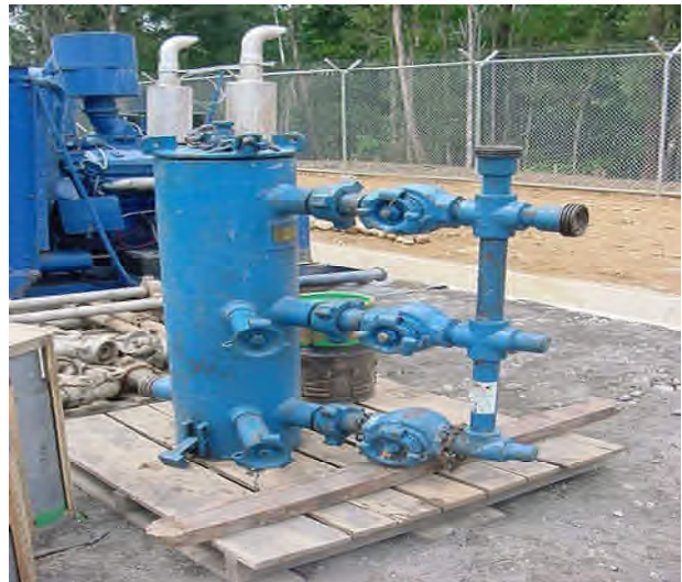
Figure II.44 : Tête de cimentation. [8]
