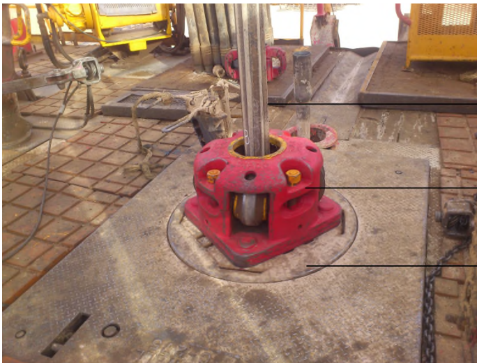
Figure II.28 : La table de rotation.
