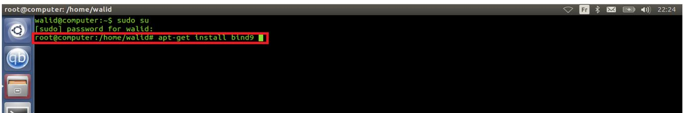
FIGURE 4.2 – Installation de bind9.
