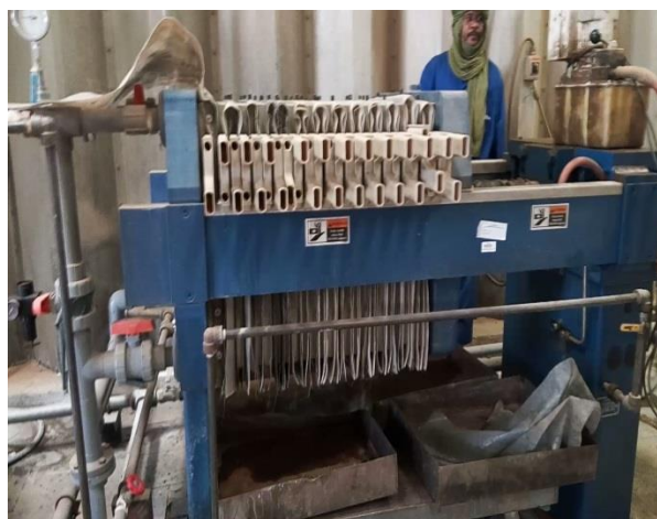
Figure II.9: Filtre Presse. [Photo prise]
