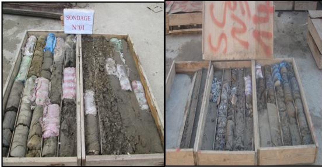
Figure II.5: Carottes issues des sondages 1 et 2 [5]
