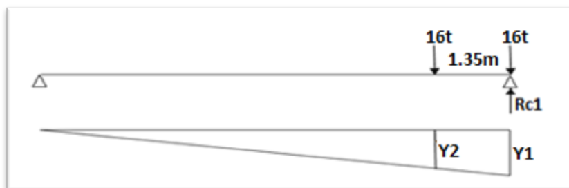
Figure III. 15: La travée sous la surcharge B_t .
