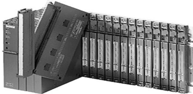
Figure II.2 : Automate type Modulaire
