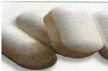
a : comprimé se collent (twinning)
