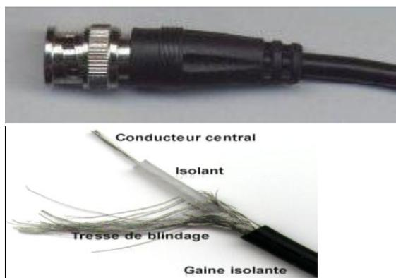
**Figure. I.1. -le câble coaxial-**
