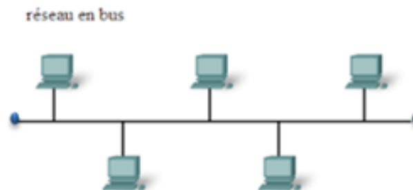
FIGURE 1.1 – Topologie en bus.
