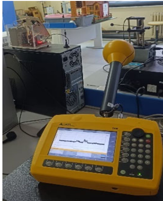
Fig. 6. Measurement setup for electromagnetic compatibility tests using SRM-3006
