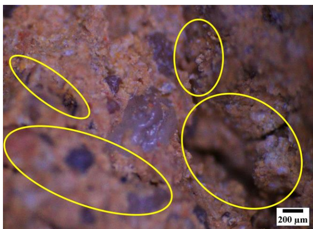
Figure 12. Earth–sand composite containing 30 wt. % olive pomace, scale: 200 μm
