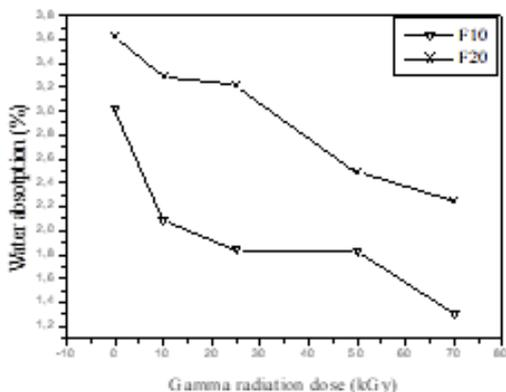
Figure 5. Water absorption of the various composites
