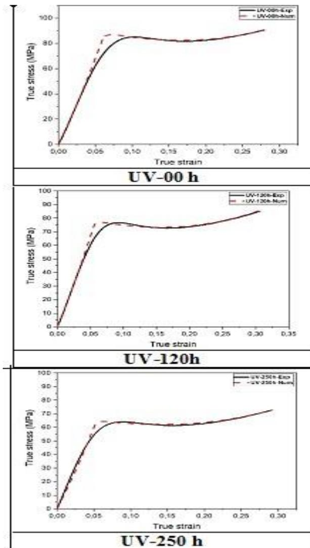
**Figure 8:** Comparison of true stress-true strain curves for each UV exposure time.
