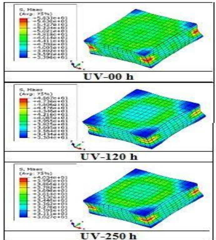
**Figure 9:** Von Mises stress distribution in the specimens after compression
