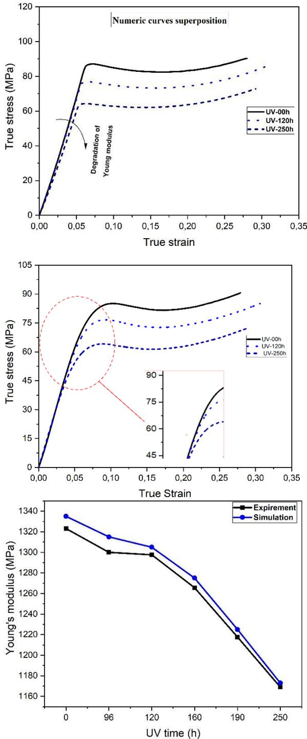
**Figure 10:** Comparing results for each holds time exposure: (a) numerical true strain-true stress curves, (b) experimental true strain-true stress curves, (c) numerical and theoretical degrading Young's modulus.
