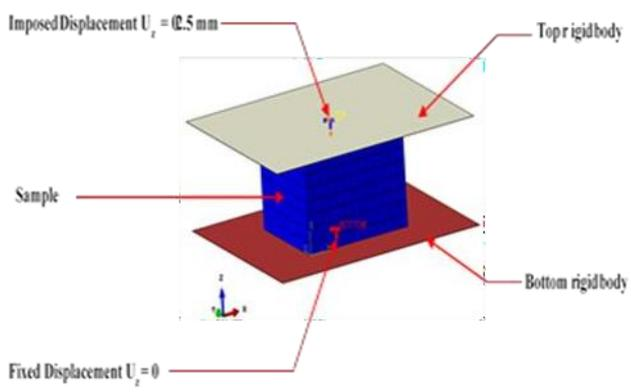
Figure 7: Boundary conditions were applied to the tested specimen
