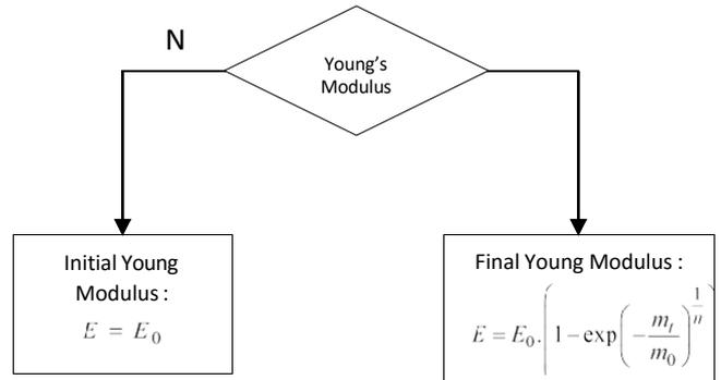
Figure: Diagram of the implementation conditions for the UV degradation
