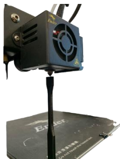
Figure 7 Printing of a specimen along the Z-axis
