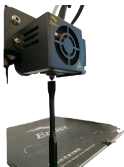
Figure 7 Printing of a specimen along the Z-axis
