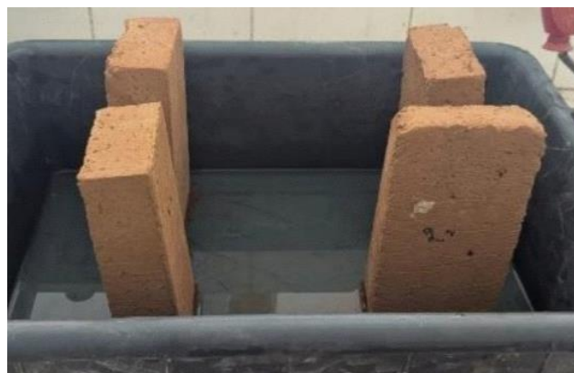
Figure 13. Capillary absorption test in accordance with standard NF EN 772-11.
