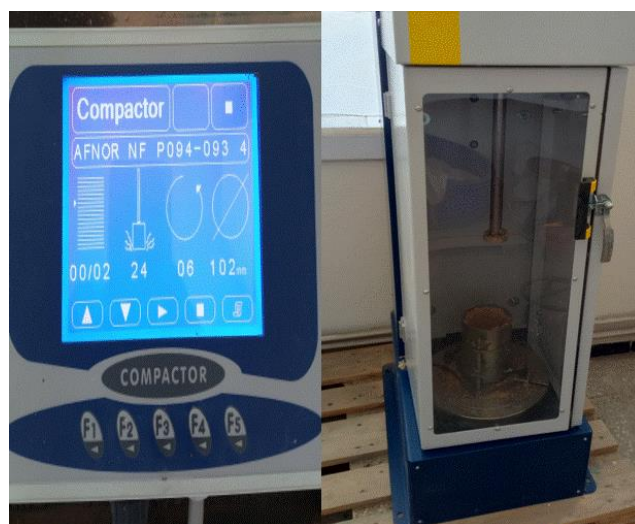
Figure 5. Experimental Setup for the Standard Proctor Test.
