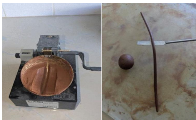
Figure 6. Casagrande Apparatus for the Atterberg Limits Test.
