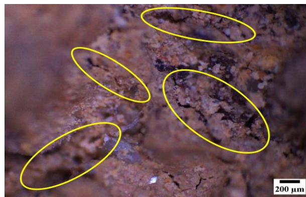
Figure 11. Earth-sand composite containing 20 wt.% olive pomace, scale: 200 μm
