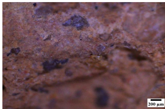
Figure 9. Optical macroscopy image showing the microstructural features of the reference composite containing 0 wt.% olive pomace, observed at a scale of 200 μm.
