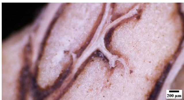
Figure 3. Olive Pomace Particles under Optical Microscope (200 μm)
