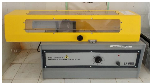
Figure 4. Sand Equivalent Test Apparatus.
