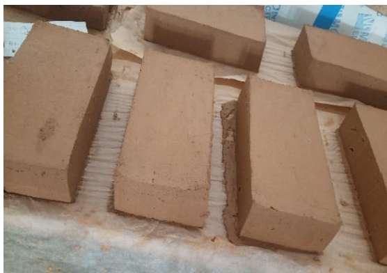
Figure 7. The prepared composite brick specimens (5 x 10 x 20 cm)
