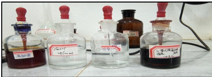
Figure III.5. Les solutions Bromophenolblue Na 2 OH HNO 3 diphenylcarbazonne (laboratoire STG cimenterie d'Adrar).
